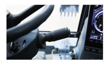
▶ Constant-speed cruise control reduces driving fatigue. Automatic oscillation locking mode meets different driving conditions.
