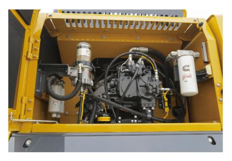
> The engine guard adopts upturning structure design, and the open angle is wide, so that it is convenient for maintenance of engine and radiator.
