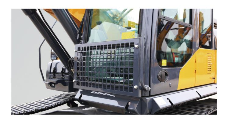
▶ ROPS certified cab can be equipped with top guard, front guard and side guard the requirements of anti-falling objects, and further improving the safety of the cab.Rear camera and right camera have better view.
