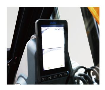
New generation of instruments: high-end 7-inch large screen display, detailed page layout, clear picture quality, reserved video display function in addition to main functions, and supporting a variety of video formats.
